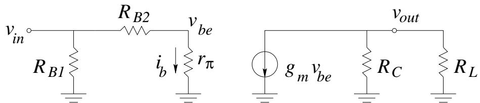
The value of the small-signal input resistance is determined by the DC base current;  $r_\pi = nV_T/I_{BQ}$ , where  $n$  is the emission coefficient. The small-signal transconductance is given by  $g_m = I_{CQ}/nV_T$ .
