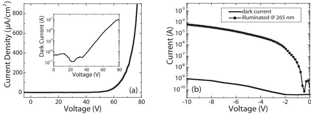
**Fig. 1** a) Dark current density of an MSM-PD with 10  $\mu\text{m}$  finger spacing. Inset shows the leakage current in logarithmic scale. b) I–V curves of a device with 5  $\mu\text{m}$  finger spacing under different illumination conditions.
