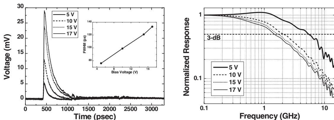
**Fig. 3** a) Bias-dependent temporal pulse responses of an AlGaIn MSM PD with 3  $\mu$ m finger spacing. Inset shows the measured FWHM values with respect to bias voltage. b) Corresponding FFT curves with 3-dB bandwidths of 5.4, 2.1, 1.7, and 1.5 GHz at 5, 10, 15, and 17 V bias respectively.
