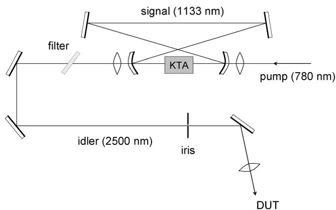
Fig. 6. Schematic diagram of the optical parametric oscillator.
