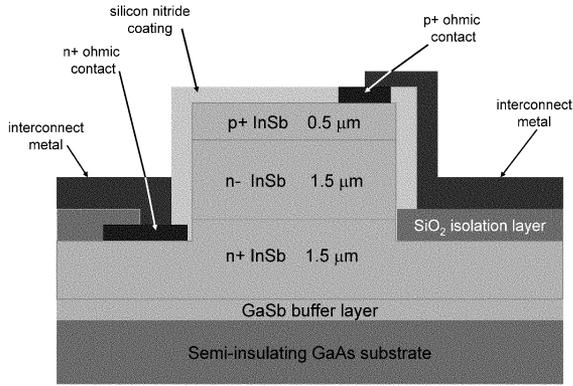
Fig. 1. Cross section of a fabricated photodetector.
