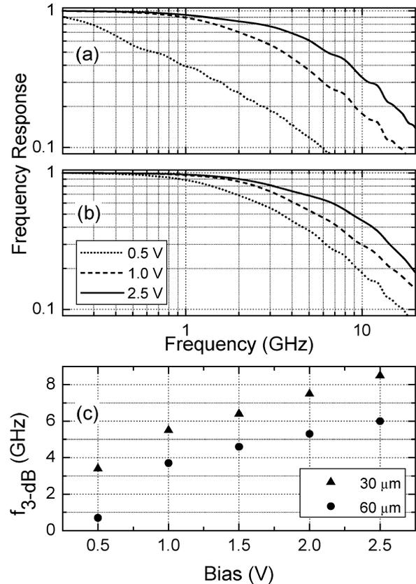
Fig. 9. FFT of the temporal responses of the photodetectors. Results for (a) 60- $\mu\text{m}$  diameter and (b) 30- $\mu\text{m}$  diameter photodetectors as a function of bias are shown. (c) 3-dB bandwidth of the 30- and 60- $\mu\text{m}$  diameter photodetectors as a function of applied bias.
