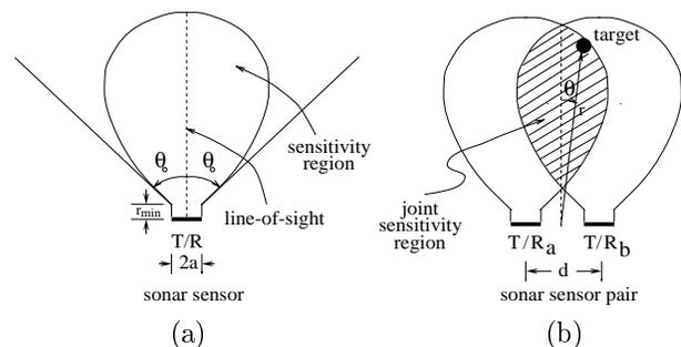
Figure 1: (a) Sensitivity region of an ultrasonic transducer. (b) The joint sensitivity region of a pair of ultrasonic transducers.
