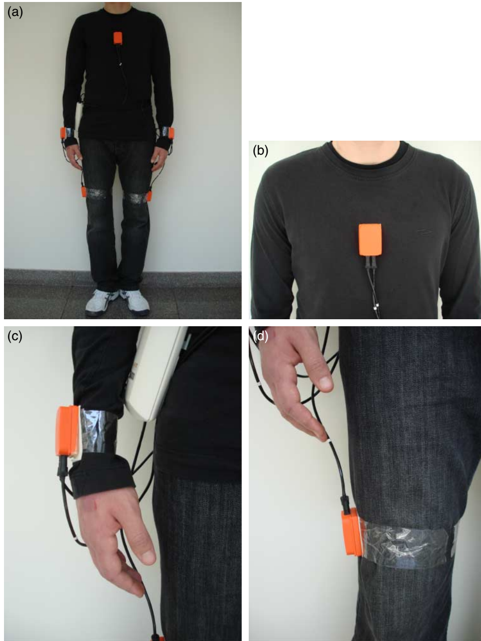
FIGURE 2. Positioning of the MTx units on the body.
