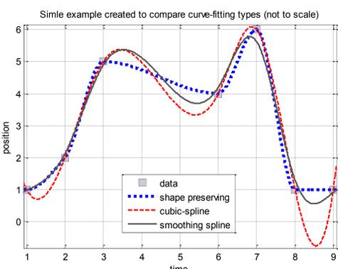
Figure 3. The three curve-fitting methods applied to simple synthetic data.
