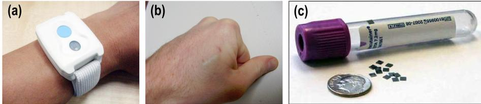
Figure 1. (a) an active RFID tag worn as a bracelet, (b) a passive RFID tag buried under the skin, (c) tiny RFID tags of size 2 × 2 mm.
