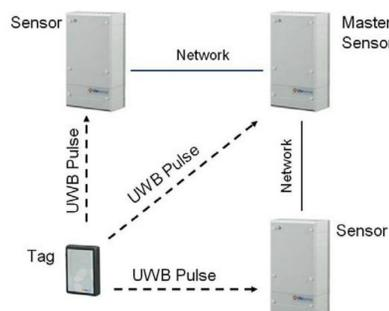
Figure 2. Ubisense hardware components.
