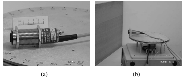
Fig. 1. (a) The IR sensor and (b) the experimental setup used in this study.
