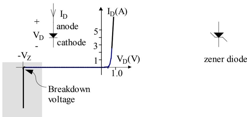
Figure 2.20 Zener diode and its characteristics
