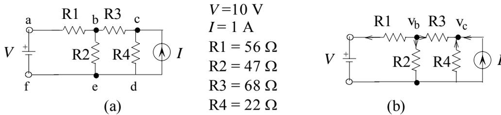
Figure 2.9 Two-node circuit
