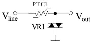
Figure 2.27 Over-voltage protection circuit
