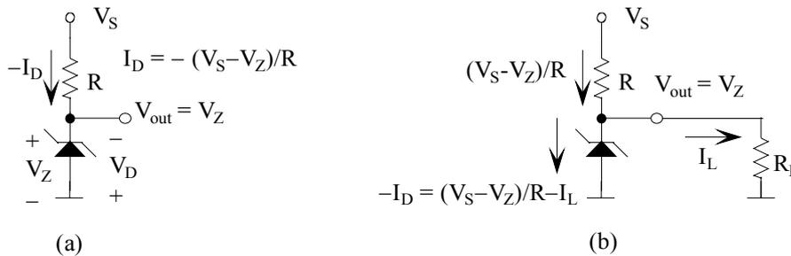
Figure 2.21 Zener diode in a voltage reference circuit
