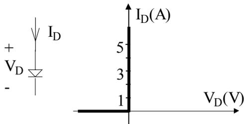
Figure 2.15 Ideal diode equivalent circuit and characteristics
