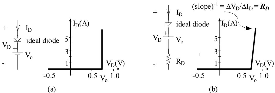
Figure 2.16 Piecewise linear diode equivalent circuits and characteristics
