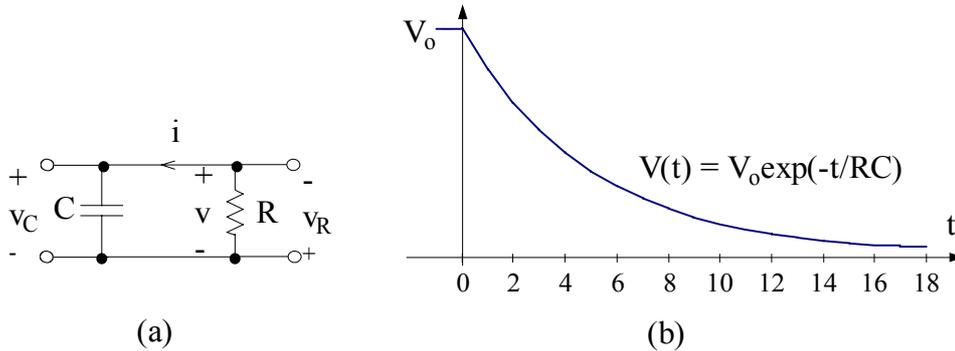
Figure 2.11 RC circuit
