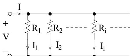
Figure 2.3 Parallel resistors
