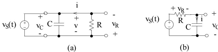
Figure 2.12 Parallel and series RC circuit
