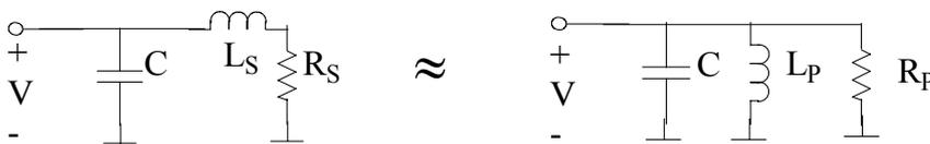
Figure 4.7 Tuned circuit with lossy inductor
