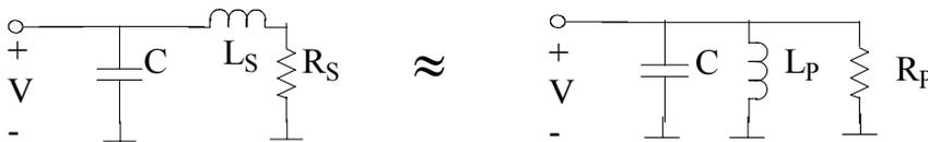
Figure 4.7 Tuned circuit with lossy inductor
