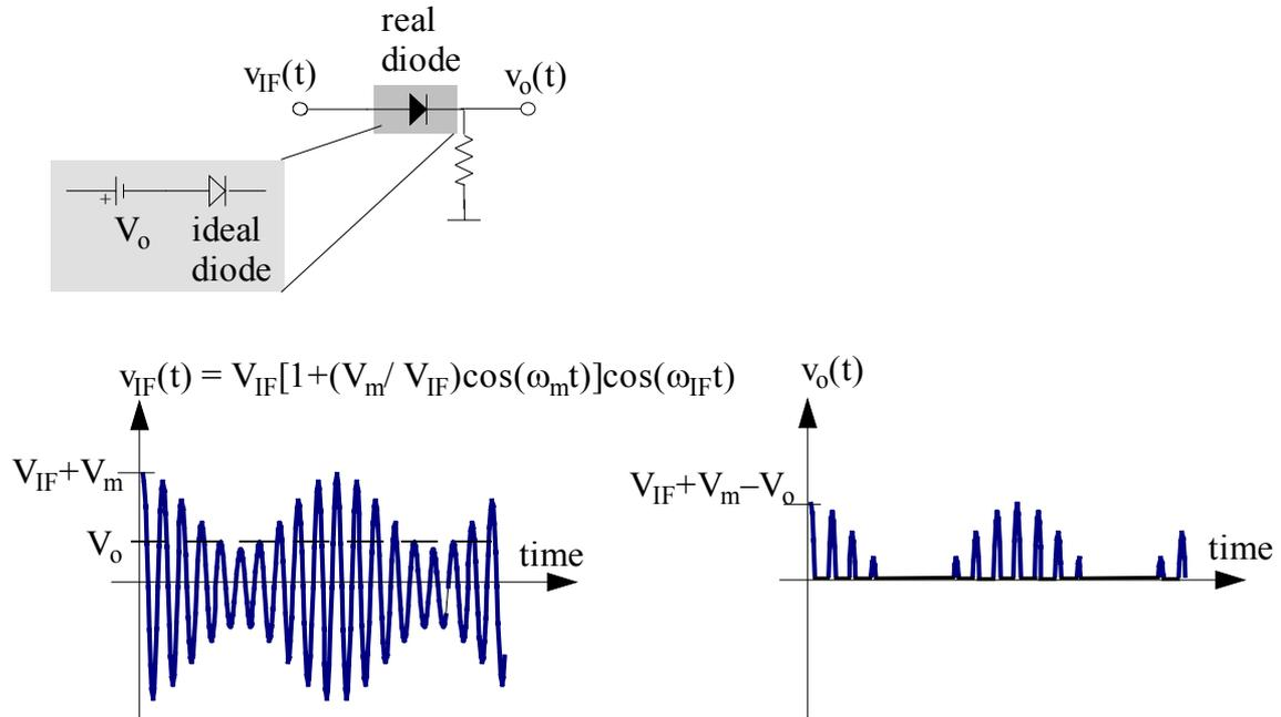
Figure 6.4 Rectifier with a real diode
