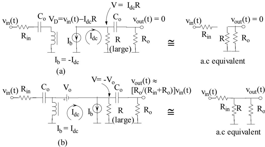
Figure 6.7 Diode switch circuit when (a)  $I_b = -I_{dc}$  and (b)  $I_b = I_{dc}$
