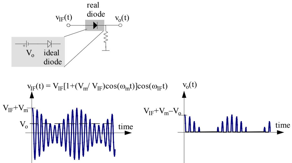
Figure 6.4 Rectifier with a real diode
