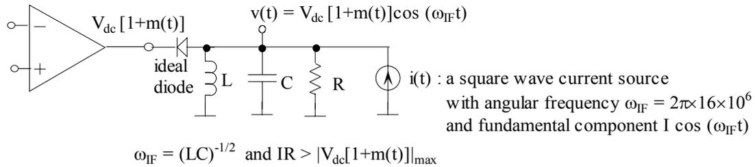
Figure 7.2 Amplitude modulator
