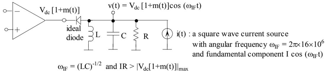
Figure 7.2 Amplitude modulator
