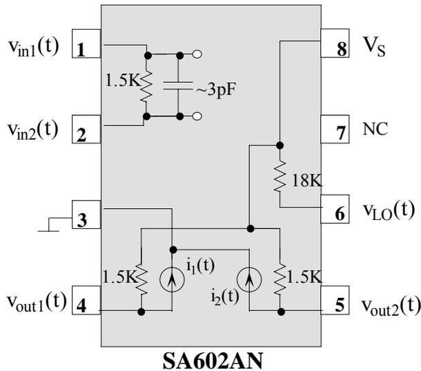
$$i_1(t) \approx (0.8 \text{ mA}) \{1 + \tanh[k(v_{in1} - v_{in2})] \times \tanh[kv_{LO}]\}$$
