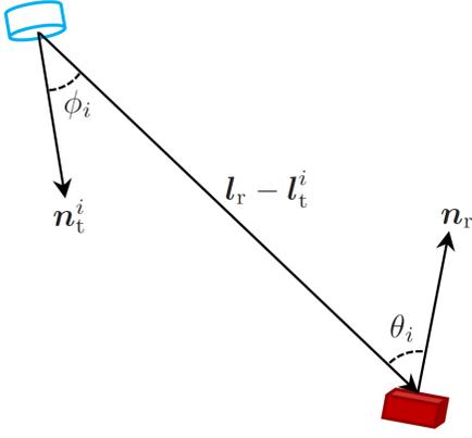
Fig. 2. Illustration of configuration parameters in the Lambertian model, where the cylinder represents the  $i$ th LED, and the rectangular prism denotes the PD.
