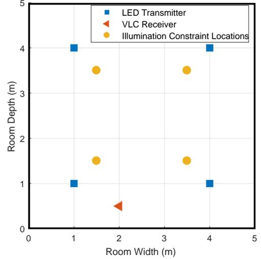
Fig. 7. VLP scenario with four LED transmitters and a VLC receiver, shown in two-dimensions.
