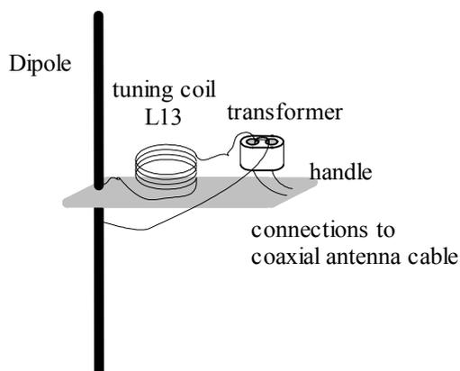
Figure 8.12 Antenna connections
