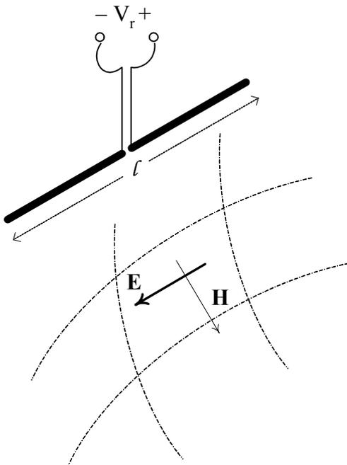
Figure 8.5 Receiving dipole
