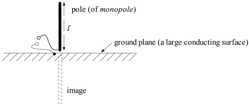
Figure 8.8 Monopole antenna
