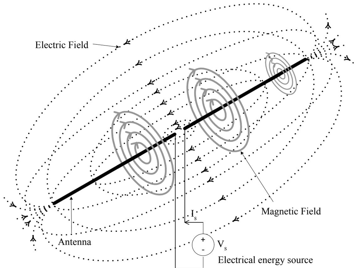
Figure 8.1 Dipole antenna and radio wave generation concept
