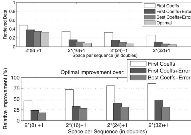
Fig. 15. Top: Ratio of uncompressed sequences retrieved from disk (smaller numbers are better). Bottom: Improvement of Optimal against all other approaches (higher numbers are better).
