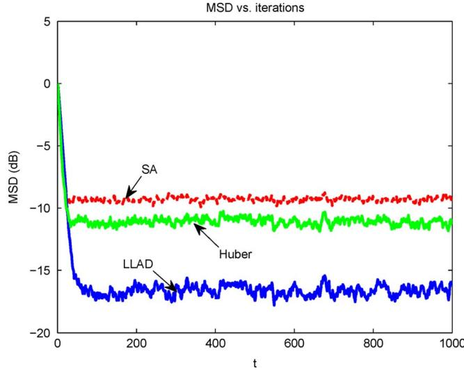
Fig. 12. Comparison of the time evolution of the MSD of the SA, robust Huber and LLAD algorithms in the 5% impulsive noise environment.
