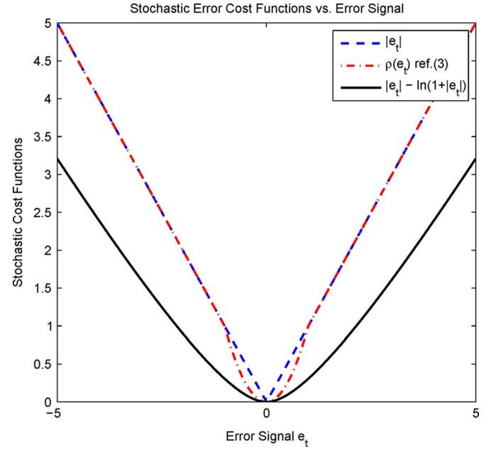
Fig. 2. A comparison of the stochastic cost functions illustrating the decreased steepness of the absolute difference algorithm in the logarithmic error cost framework for relatively small error.
