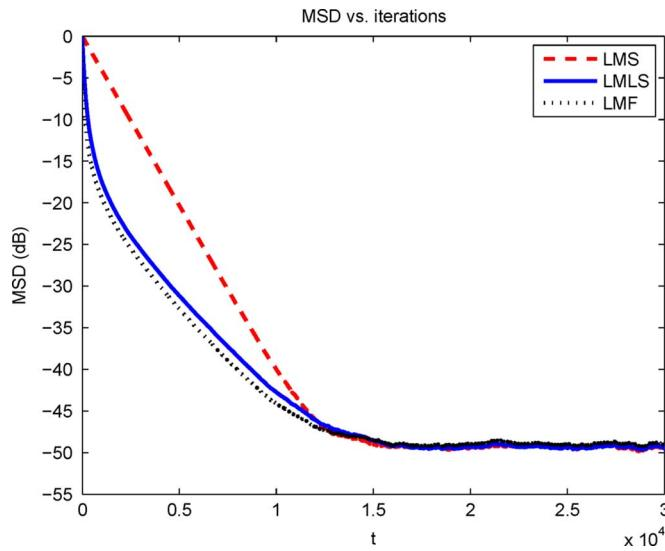
Fig. 6. Comparison of the MSD of the LMLS, LMS and LMF algorithms for the same steady-state MSD where  $\mu_{\text{LMLS}} = \mu_{\text{LMF}} = 0.01$  and  $\mu_{\text{LMS}} = 0.00047$ .
