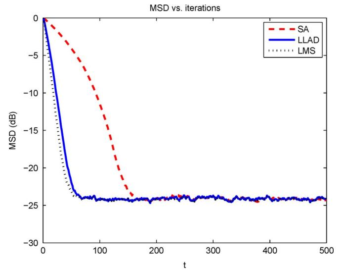
Fig. 8. Comparison of the MSD of the LLAD, SA and LMS algorithms in impulse-free noise environment with  $\mu_{\text{LLAD}} = 0.12$ ,  $\mu_{\text{SA}} = 0.01$  and  $\mu_{\text{LMS}} = 0.1$ .
