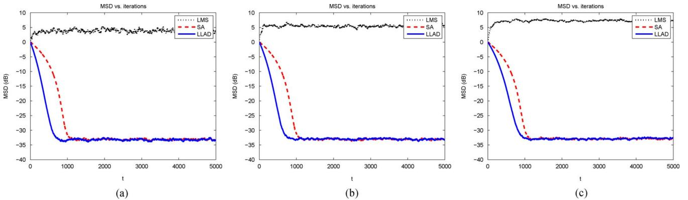
Fig. 10. Comparison of the MSD of the LLAD, SA and LMS algorithms in 1%, 2% and 5% impulsive noise environments. (a) 1% ( $\alpha_{\text{opt}} = 1.005$ ), (b) 2% ( $\alpha_{\text{opt}} = 1.4286$ ), (c) 5% ( $\alpha_{\text{opt}} = 2.2942$ ).
