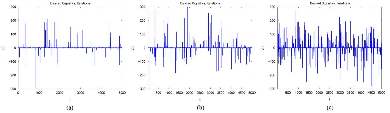
Fig. 9. Desired signal in 1%, 2% and 5% impulsive noise environments. (a) 1%, (b) 2%, (c) 5%.
