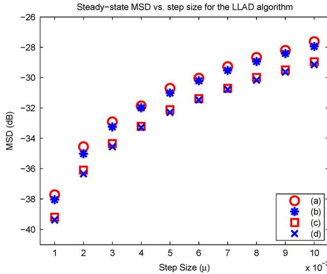
Fig. 5. Dependence of the steady-state MSD on the step size  $\mu$  for the LLAD algorithm in the 5% impulsive noise environment where (a), (b), (c), and (d) denote  $\alpha = 1$  (simulation),  $\alpha = 1$  (theory),  $\alpha_{\text{opt}} = 2.2942$  (simulation), and  $\alpha_{\text{opt}} = 2.2942$  (theory) cases, respectively.
