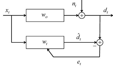
Fig. 1. Generic system identification framework.
