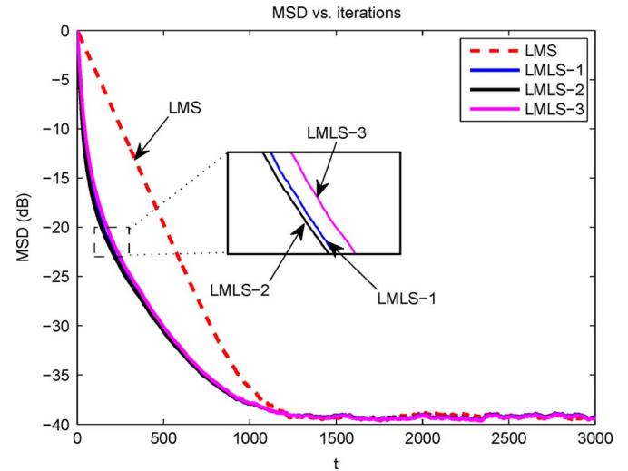
Fig. 7. Comparison of the MSD of the LMLS algorithms with different  $\alpha$ 's and the LMS algorithm for the same steady-state MSD where  $\mu_{\text{LMLS}} = 0.1$  and  $\mu_{\text{LMS}} = 0.0047$ . LMLS-1, LMLS-2 and LMLS-3 correspond to  $\alpha = 1$ ,  $\alpha = 2$  and  $\alpha = 0.5$ , respectively.
