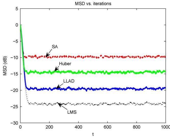
Fig. 11. Comparison of the time evolution of the MSD of the SA, robust Huber, LLAD and LMS algorithms in the impulse-free noise environment.
