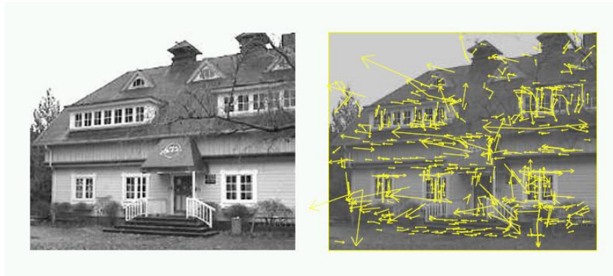
Figure 2.4: SIFT features on a sample image represented with their scales, orientations and locations [42].
