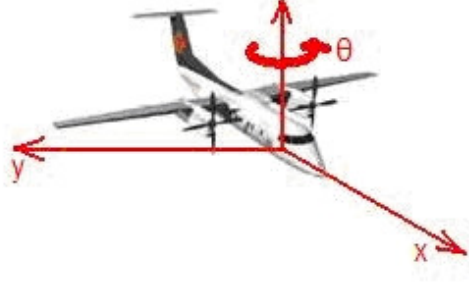
Figure 2.3: Three degrees of freedom for the process model [37].
