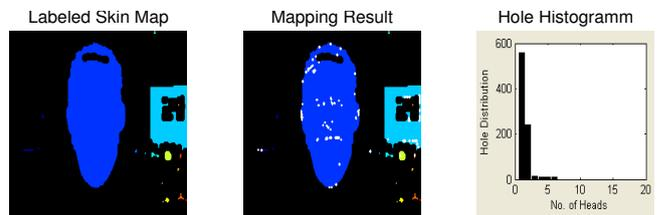
Figure 3: Hole mapping onto the labeled skin map and corresponding histogram (hole distribution).
