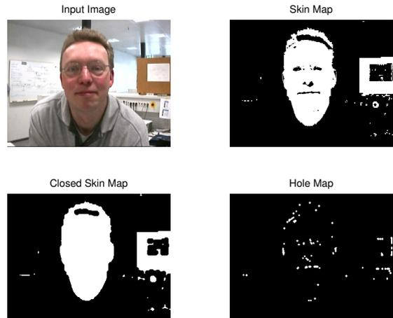
Figure 2: Illustration of the hole map generation. The hole map is computed according to Eq. 1.
