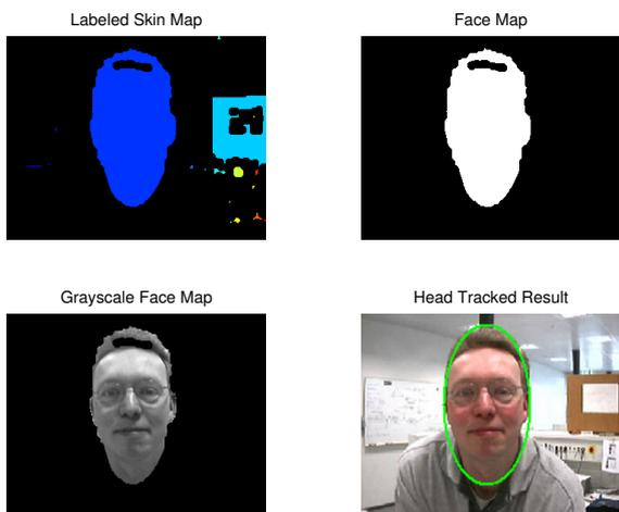
Figure 4: Face map generation by hole mapping. The textured version (lower left) was computed according to Eq. 2.
