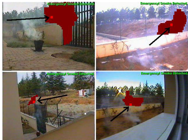
Figure 4: Sample images from test videos. Smoke regions are successfully detected. Edge points satisfying all the conditions defined by the method are marked.
