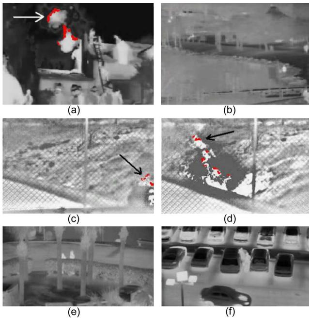
**Fig. 8** Image frames from some of the test clips. (a), (c), and (d) show fire regions detected and flame boundaries marked with arrows. No false alarms are issued for ordinary moving bright objects in (b), (e), and (f).
