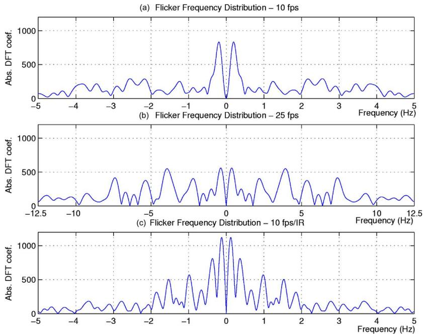
**Fig. 6** Flicker frequency distributions for (a) 10-fps color video, (b) 25-fps color video, and (c) 10-fps IR video. These frequency distributions were obtained by analyzing the temporal variations in the red channel value of a pixel at the boundary of a flame region in color-video clips recorded at 10 and 25 fps, and intensity value of a pixel at the boundary of a flame region in an IR video clip recorded at 10 fps, respectively.
