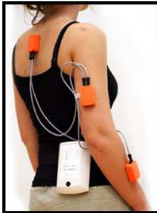
Figure 1.3: Miniature inertial sensor units worn on the body (reprinted from http://www.xsens.com/en/movement-science/xbus-kit ).
