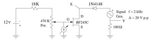
Generate and plot the  $i_D$  vs  $v_{DS}$  curve for  $V_{GS}=0, -1, -2, -3, -4, -5, -6, -7$  V. Measure  $I_{DSS}$  by noting the saturation current when  $V_{GS}=0$  V. To measure  $V_p$ , set  $V_{GS}$  close to where  $I_D \simeq 0$  and change the 100  $\Omega$  resistor with a 10 K $\Omega$  resistor. Then slowly adjust  $V_{GS}$  to determine when  $I_D$  becomes exactly zero to find  $V_p$ .
