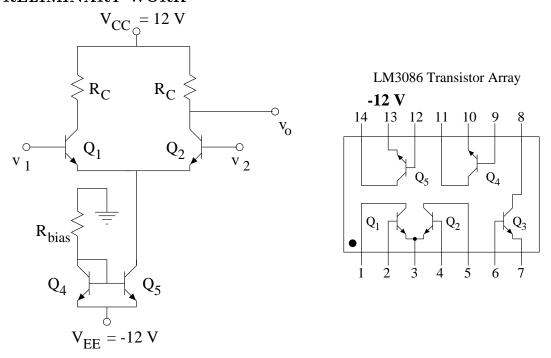
1. Design a differential amplifier biased by a current source based on the circuit topology given in the figure. You will use the integrated circuit transistor array LM3086 whose connection diagram is shown in the same figure. For each transistor on this IC, you can assume that  $\beta = 100$  and  $V_A = 50$ .
