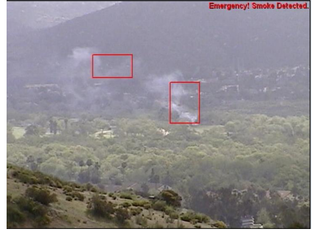
Fig. 5. A snapshot from an independent test of the system by the Regional Technology Clearing House of San Diego State University in California in April 2009. The system successfully detected the test fire and did not produce any false alarms. The detected smoke regions are marked with rectangles.
