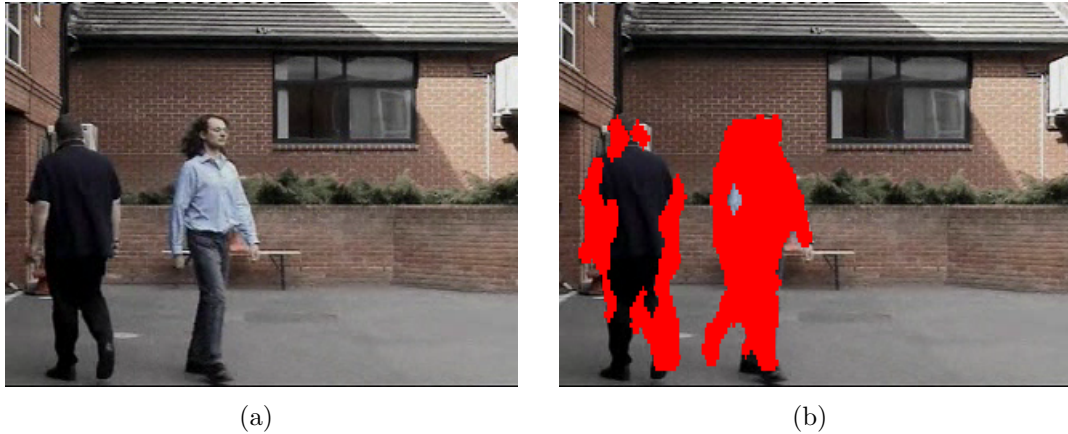
Figure 2.2: Temporal differencing sample. (a) A sample scene with two moving objects. (b) Temporal differencing fails to detect all moving pixels of the object on the left hand side since it is uniform colored. The detected moving regions are marked with red pixels.
